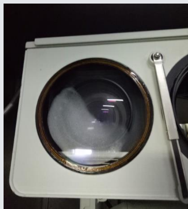
IPX5/IPX6 flush test
